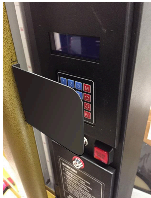
Opening of the main door for service exposes the keypad, enabling password entry.
